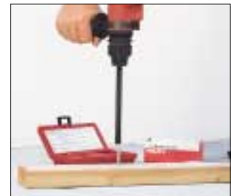
Adjust the depth location and set the screw.
