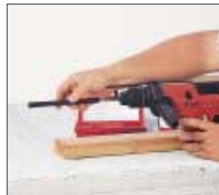
Change the rotary hammer setting to rotation only. Lock the compact setting tool over the special detent receiver on the bit.
